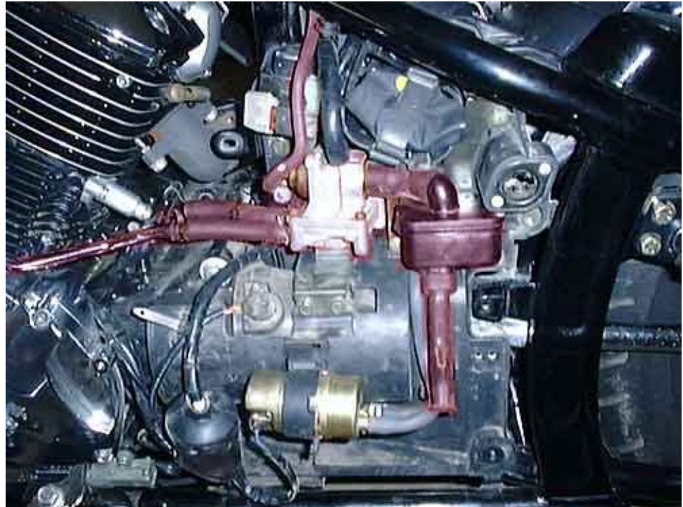
Covers removed. AIS assembly highlighted in red.
