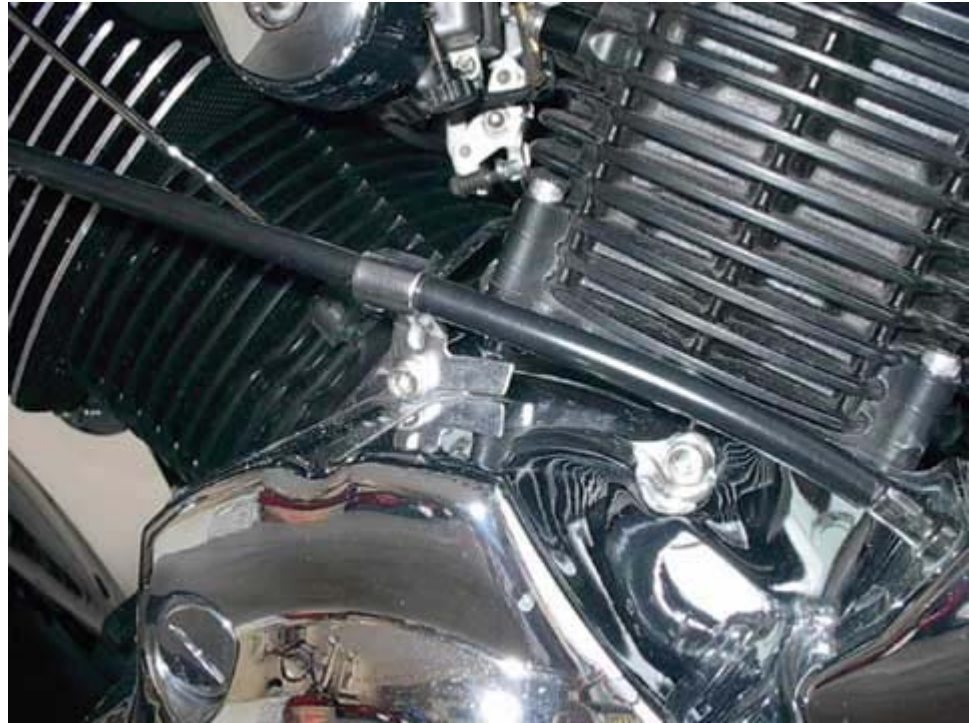
Cut, smooth and then replace the Clutch Cable Bracket.
