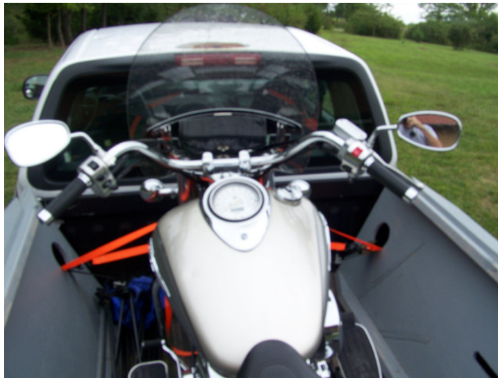
Fig 2. Bike is loaded and ready to transport. Notice the tie-down straps passing thru the holes in the disassembled ramp sections along side the bike. The straps attach to anchor points on the truck bed behind the ramp sections.
