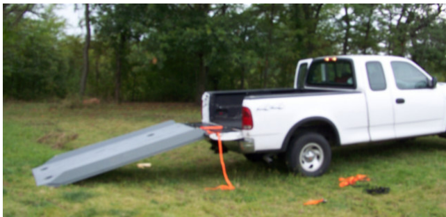
Fig 5. Here you get a better look at the 1" x 6" guard rails that remove some anxiety about sliding off the edge. Actually, with the sand-finish paint the tires gripped well and never slipped or spun, even when I loaded the bike in a driving rain (no, I didn't stop to take pictures of that fiasco).
