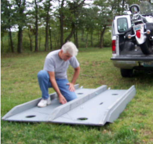
Support the center of the two ramp sections to better align the bolt holes
