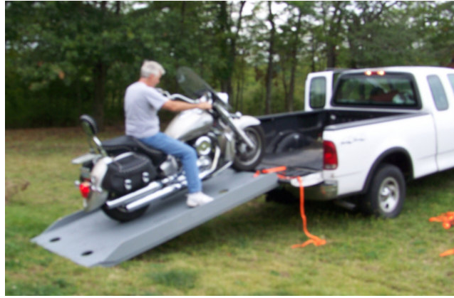
Fig 1. Unloading the bike. Notice the orange ratchet strap holding the ramp tight to the tail gate. Also, the rear wheels of the truck are in a shallow swale and the truck is facing slightly uphill for a little gravity assist in unloading.
