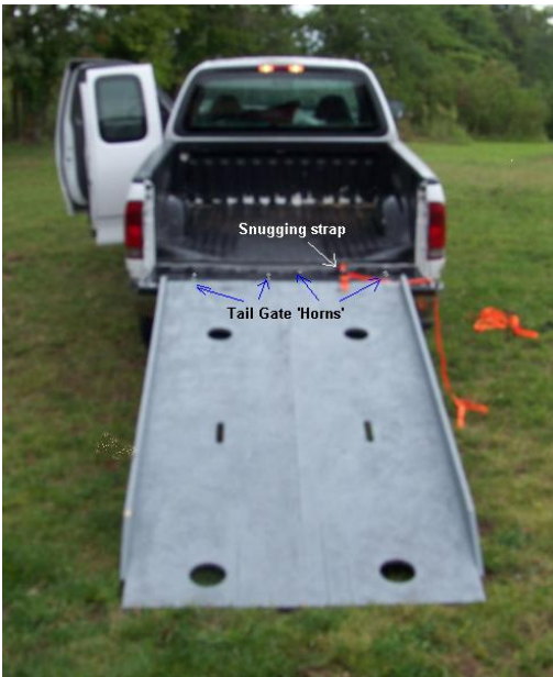
Fig. 4 The ramp is assembled and secured to the tail gate. You can see the 5" tie down strap pass-thru holes, the hand grip slot in the center of each section and (barely) the ratchet strap slots that the orange strap is passing through to secure the ramp to the tail gate.
