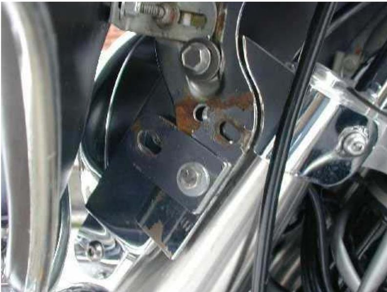
I had to clamp the little add ons into place, as there’s no way to get the bolts through until you’ve removed the fairing from the bike. You can then mark everything for drilling from behind again and pull the fairing off. I drilled and fitted my add-on brackets, bolted them into place and then test fit the while thing one more time. (see Pic 3) As you can see I had a little more work to do yet to get nice ninety-degree angles on the joints.
