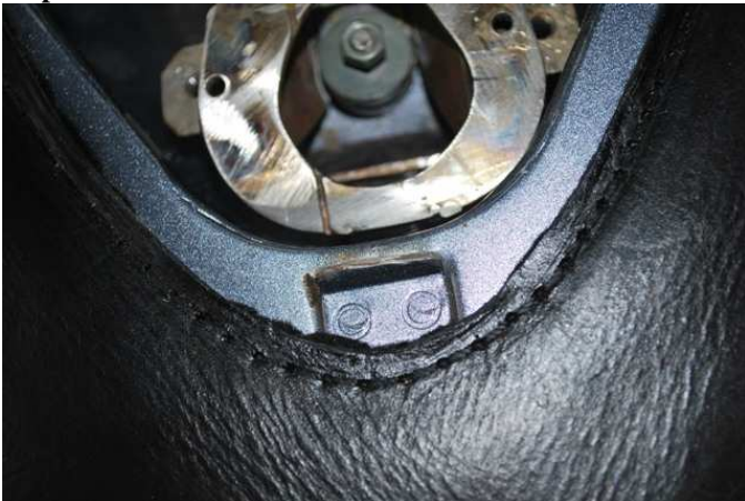
Tank tab removal
