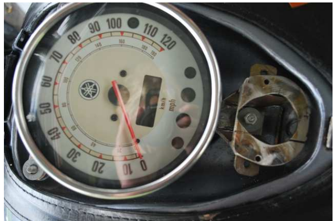
Ignition switch bracket in position
