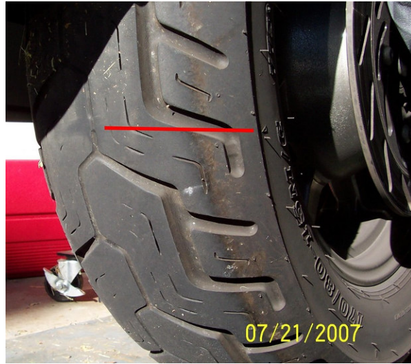
Wear bar in relation to sidewall tread wear indicator
