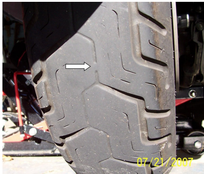
Wear bar in centre groove with a tread depth of 2/32" or less
