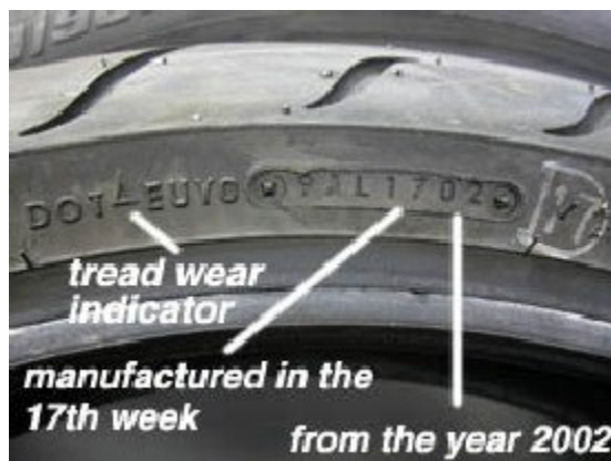
Sidewall tread wear indicator
